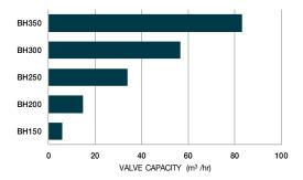
Anval BH Series valves are best suited for food, flour, grains, plastic, chemical, pharma, and milling industries. BH Series rotor is fabricated open-ended style, perfectly designed and manufactured to have a close radial clearance of 0.10 mm.
